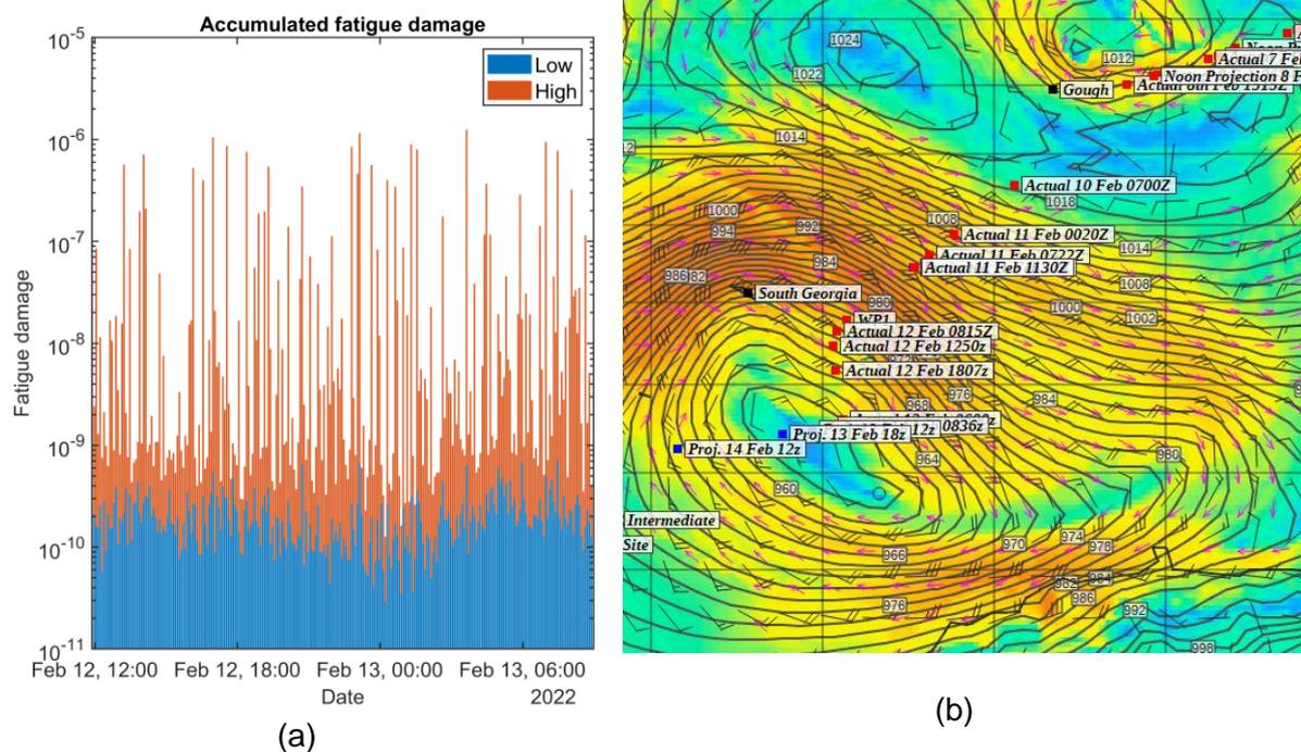
**Figure 70:** (a) A sample analysis of high and low frequency fatigue damage in the context of the (b) open water transit of the SAII on 13 February 2022 (Courtesy of the South African Weather Service).
