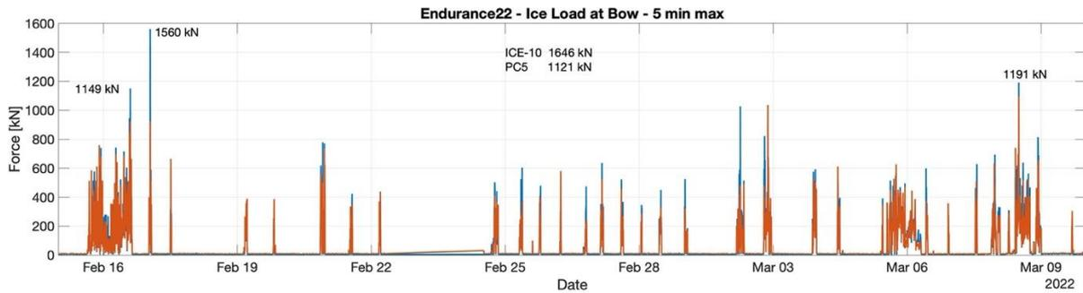
**Figure 63:** The ice loads measured from two frames at the bow. Also shown are the design ice loads for PC5 and ICE-10.
