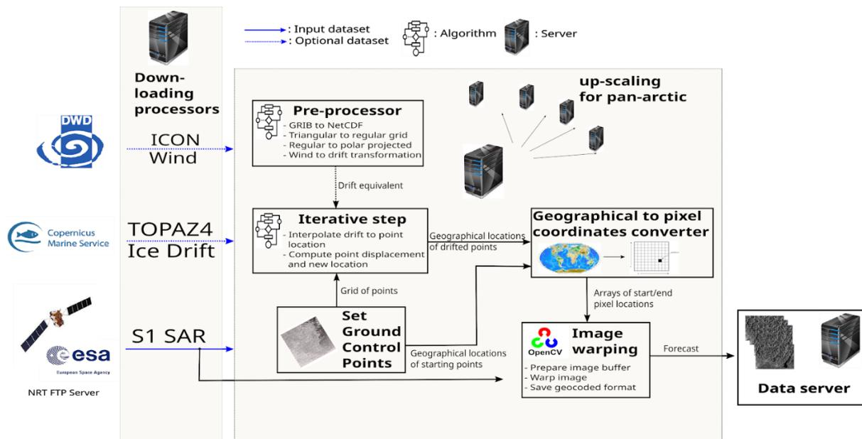
**Figure 29:** PRIIMA system architecture
