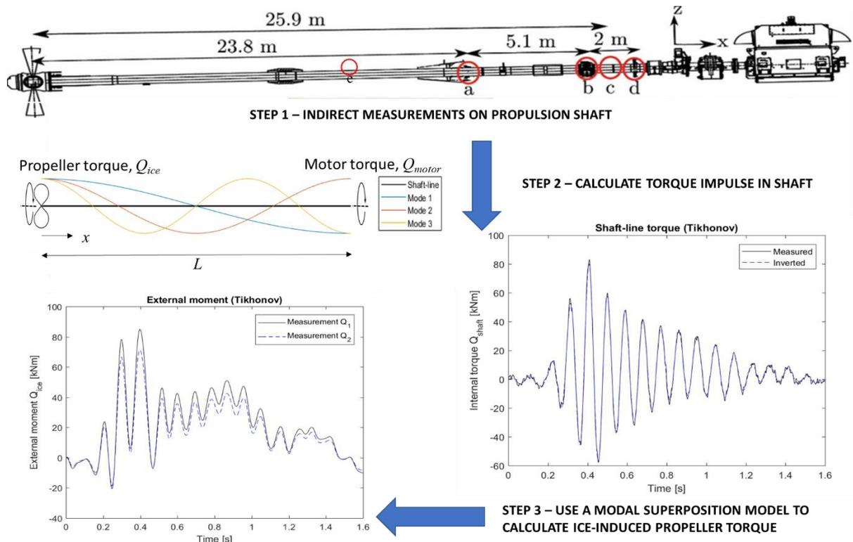
**Figure 57:** A diagram depicting the methods involved with determining the inverse-ice-induced propeller moment.
