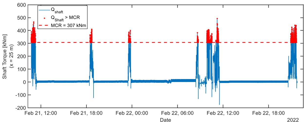
**Figure 58:** Port side shaft torque of the SA Agulhas II during ice navigation in the Weddell Sea. The values are reflected against the maximum continuous rating of the shaft.
