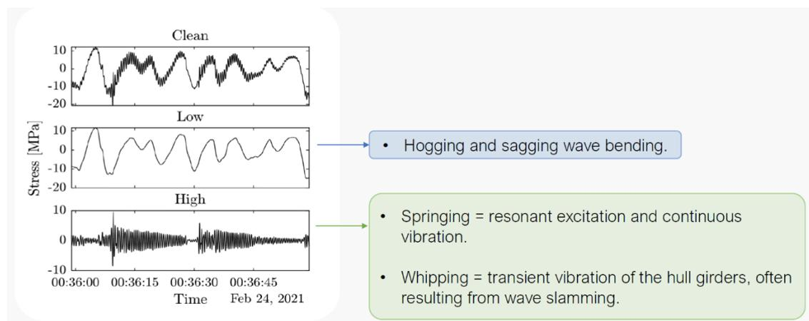
**Figure 69:** The high and low frequency components of fatigue.
