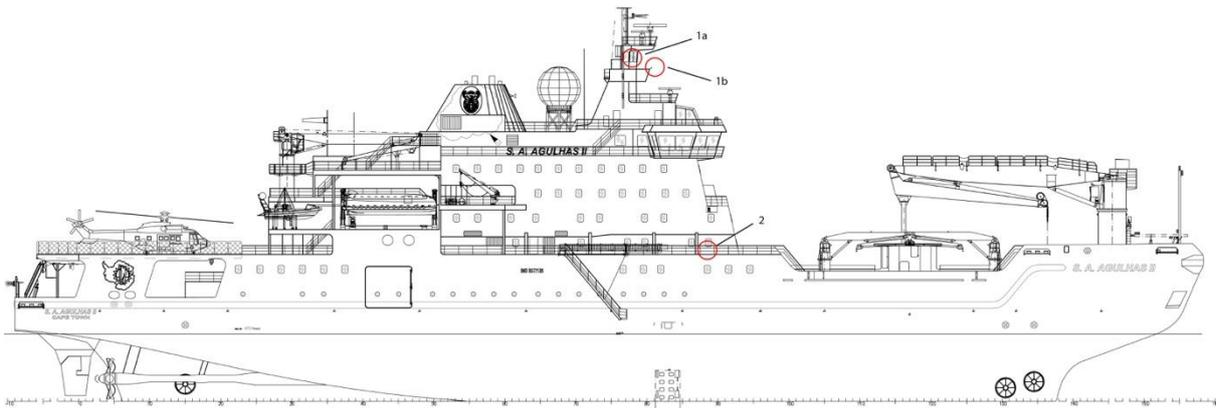
**Figure 39:** The crow's nest (1a) was used to operate a camera (1b) looking forward. Another camera (2) was looking at the ice broken by the ship bow.
