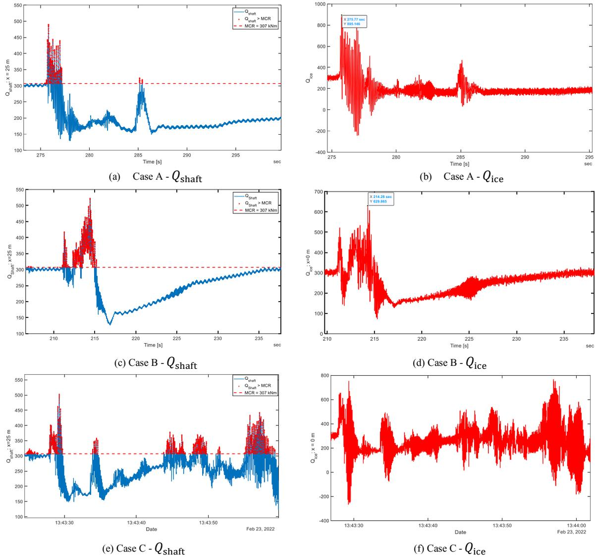
**Figure 59:** Examples of shaft torque measurements and ice-induced propeller moment calculations.
