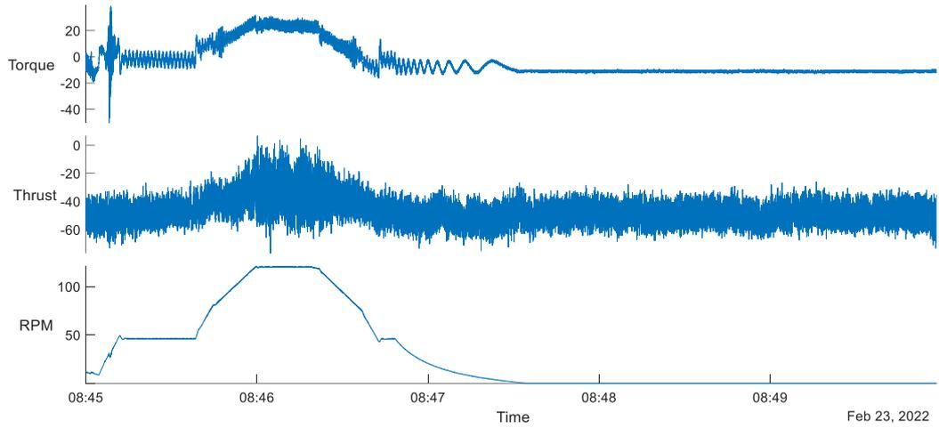
(a) Torque, thrust and rpm of the port side propulsion shaft.
