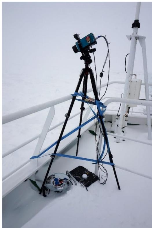
**Figure 43.** Photo of the infrared camera set up. The camera is set at 30 deg angle to the horizon.
