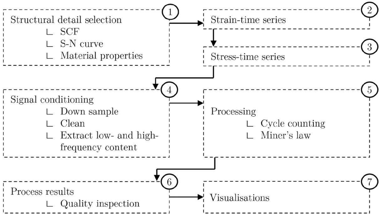
**Figure 66:** Steps of the full-scale fatigue calculation.
