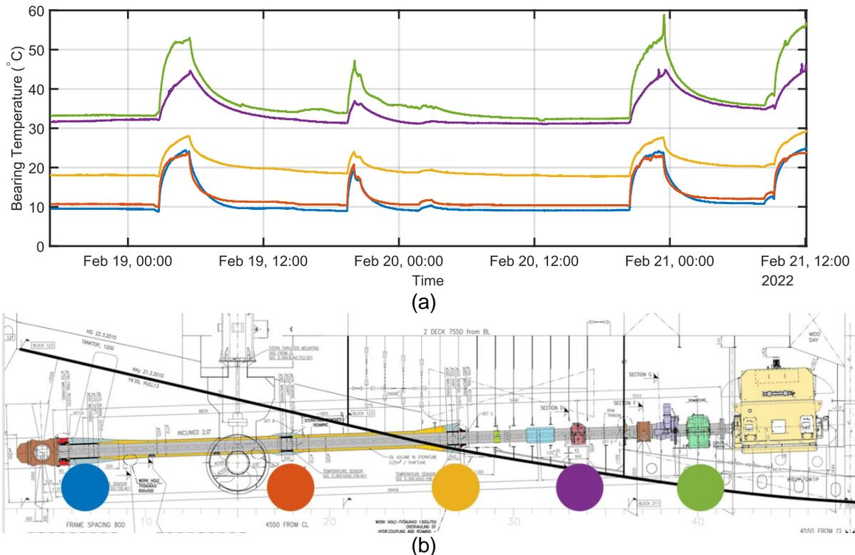
**Figure 60:** Preliminary results from bearing measurements on five bearings along the port side shaft of the SAAll during ice navigation.
