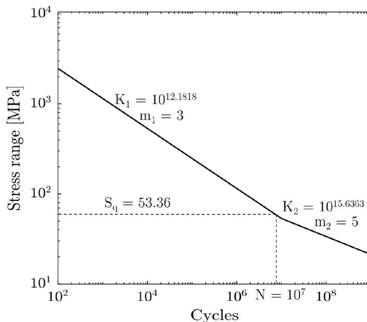
**Figure 68:** A S-N curve for steel welded joints in air plotted on logarithmic axes.
