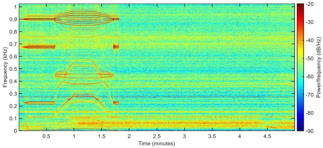
(b) A spectrogram of the acceleration on the motor housing.
