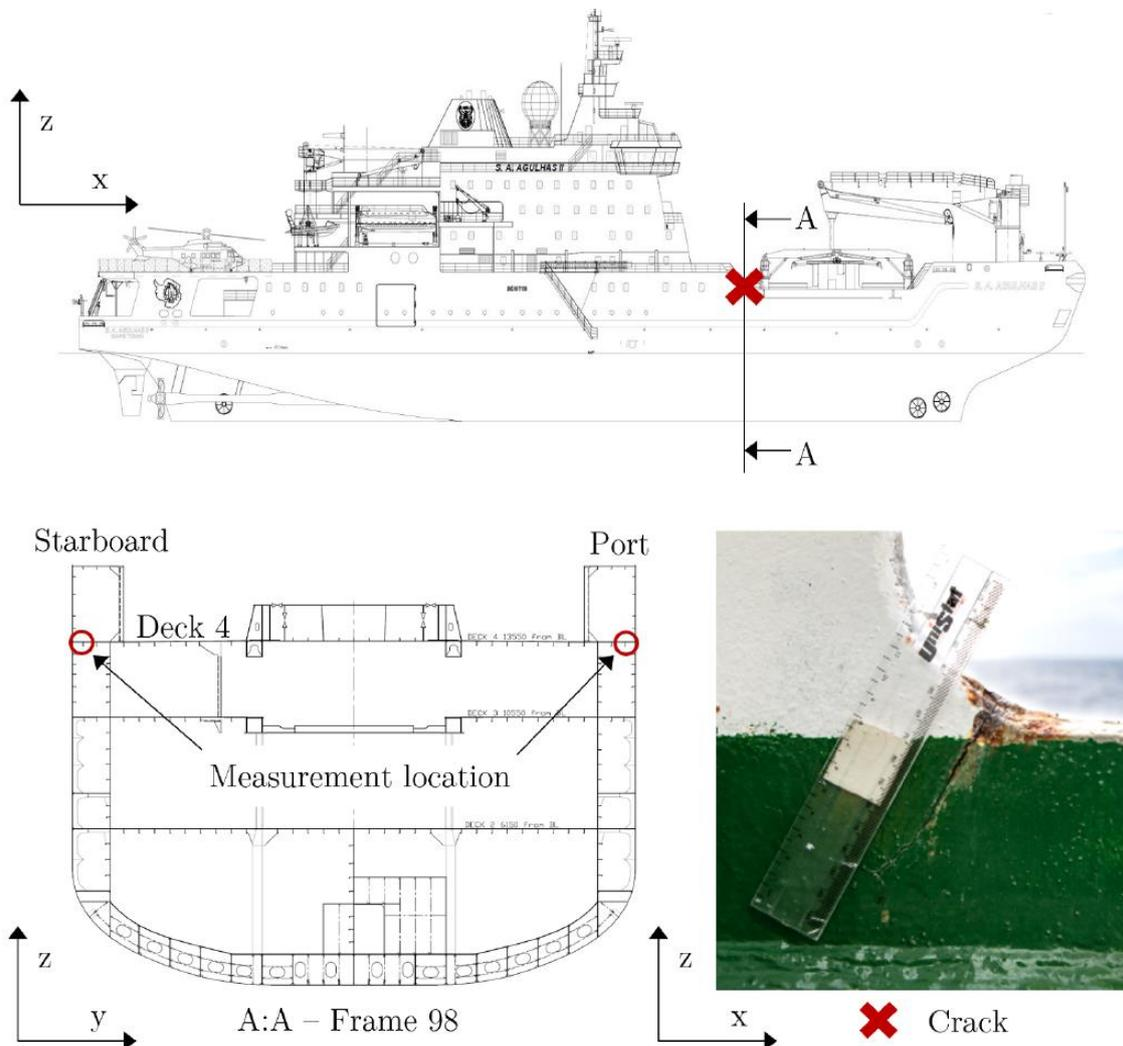
**Figure 65:** Strain measurement locations and nearby cracking.
