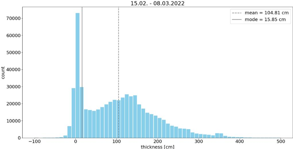
**Figure 48:** The ice thickness distribution measured by a shipborne EM instrument during the Endurance 22 Expedition
