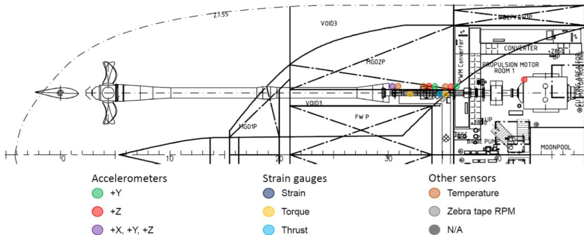
**Figure 56** Overview of measurement infrastructure on the port side shaft of SAAII.
