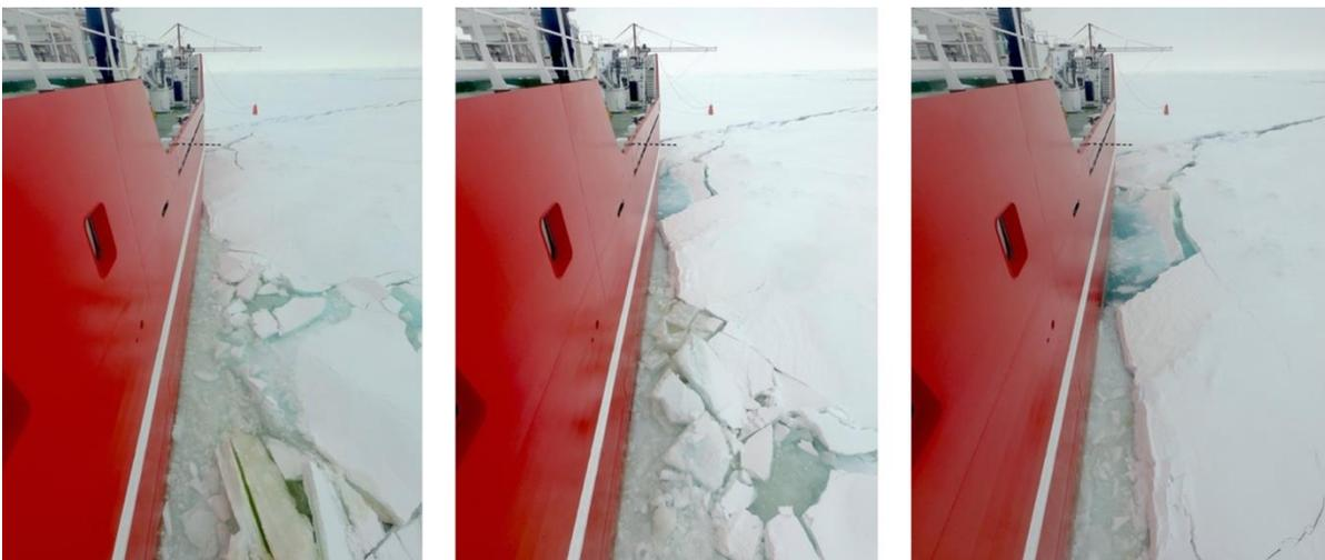
**Figure 41:** A sequence of images showing the ice failure process at the SB side of the ship bow.
