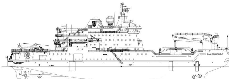
**Figure 62:** SA Agulhas II. The three rectangles on the hull show locations where ice loads are measured.
