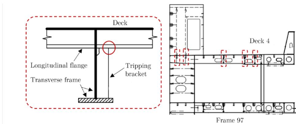
**Figure 67:** Longitudinal deck stiffener to a transverse web frame connection.
