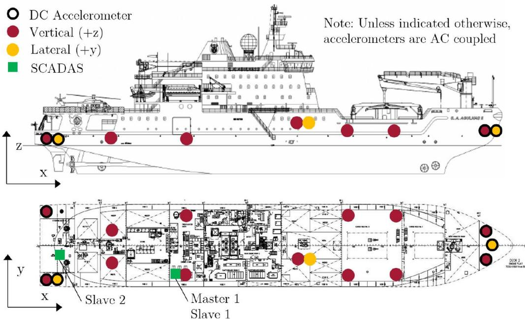
**Figure 64:** Overview of accelerometer measurements throughout the hull structure of the SAII.
